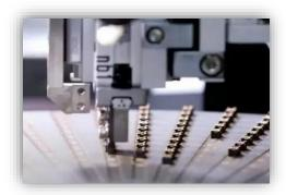
Assembling process is a step that involves integrating the wound coil and housing into a finished common mode choke. The automatic assembling process begins with preparing the coil, which is the magnetic core with wounded copper wire, followed by gluing, adhesives are used to assemble the coil and the housing with camera to control gluing position and area. After assembling the common mode choke are cured with high temperature to harden the adhesives and form a strong bond strength.
