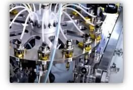
**Testing and Packing** are the final stages for ensuring all common mode chokes meet quality standards and are ready for shipment. Products are first marked by laser, and then the 100% electrical characteristics are tested, including RDC, L and SDS value with data collection, and finally packaged into carrier tape.
